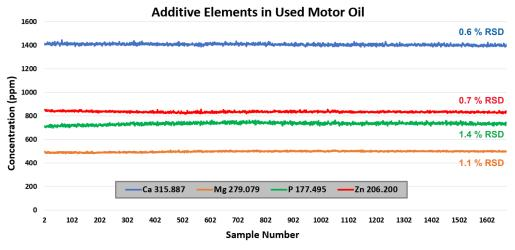
SampleSense *FAST* UHT-O System 11+ hour stability run on iCAP PRO XPS for 4 additive elements.
